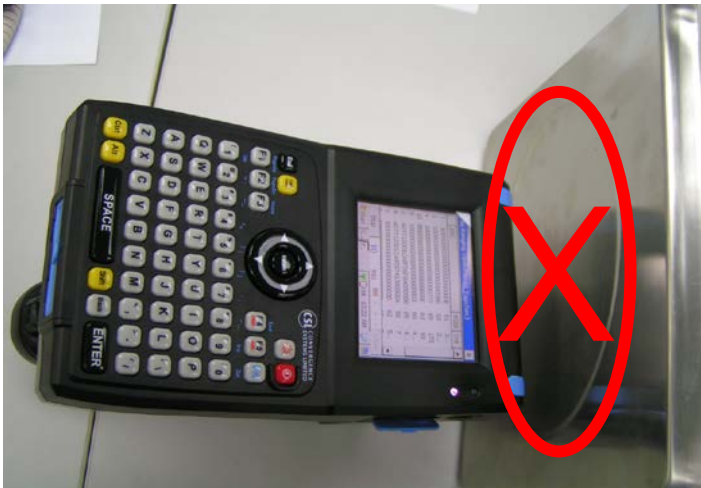
Reader antenna too close to metal
