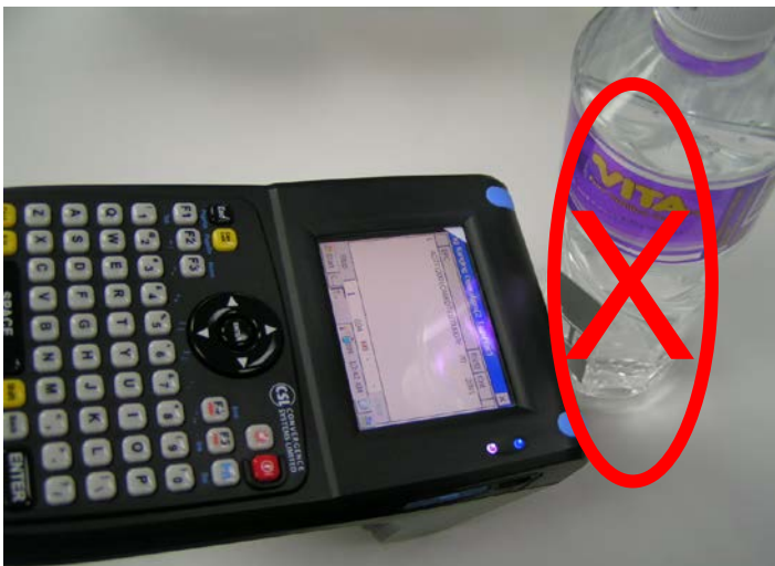
Reader antenna too close to the tag
